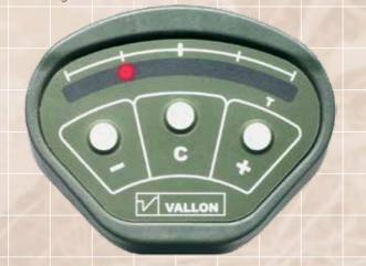
According to the polarity of the magnetic inhomogenity, the LED-signal is shifted to the left or to the right side. The position of the LED is proportional to the strength of the detection signal.
