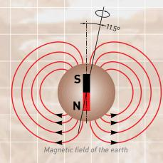
The magnetic field of the earth is homogeneous with regards to the field strength and the direction of the field strength. If a ferromagnetic object is brought into this homogeneous field, the own field of the object is superposing the local homogeneous magnetic field of the earth.
